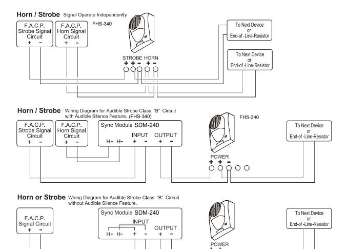
Refer to the SDM-240 Sync Module instruction manual for Class "A" wiring or other application diagrams.
